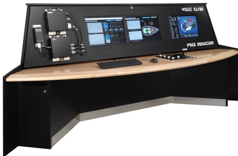
Engine virtual test bench WESTT CS/BV developed by Price Induction
